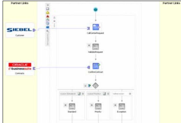
Figure 5: Oracle BPEL Process Manager orchestrating process across Siebel CRM and E-Business Suite
